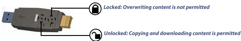
Figure 9: The PMCS Memory Key.
